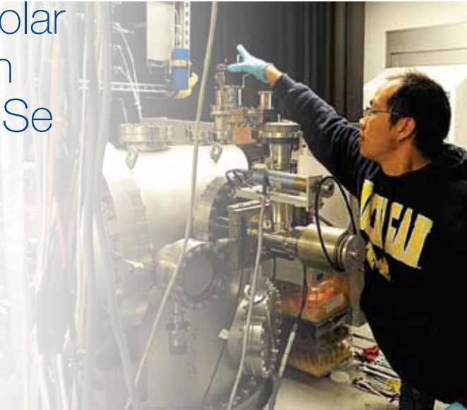
Weiming Wang growing II-VI compound semiconductor materials by molecular beam epitaxy.
