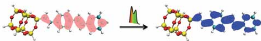
Figure 2. A plot of a silsesquioxane molecule demonstrating how the shape and location of the molecular orbitals (in pink and blue) change to include involvement with the SQ cage upon absorption of a photon of light. This reorganization of charge density implies the prospect of using molecular functionalization to improve charge separation efficiency in silsesquioxanes.
